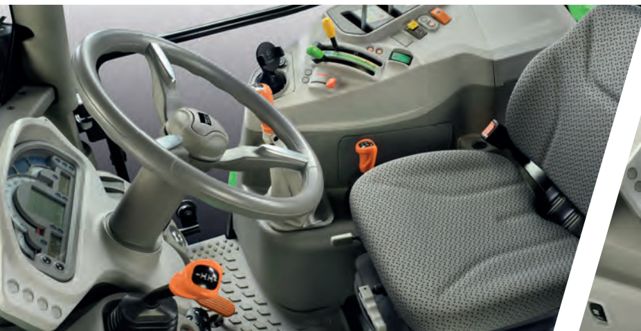
> Mechanical shuttle with ergonomic lever on steering column.
