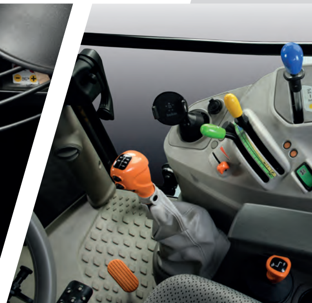
> Ergonomic and organised side control with mechanical rear lift for models 5095 - 5105 - 5105 HD.
